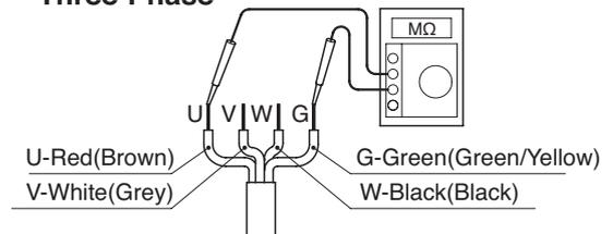
**Note:** *The insulation resistance reference value of 20MΩ minimum is based on a new or repaired pump. For reference values of a pump that has already been put into operation, refer to "7. Maintenance and Inspection" of this manual.*
